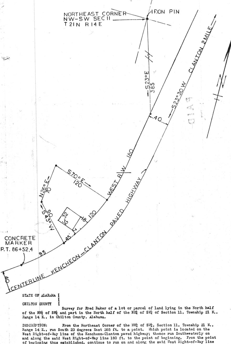
of beginning thus established, continue to run on and along the said West Right-of-Way line 120 ft. to a point; thence run South 43 degrees West 90 ft. to a point; thence run North 26
