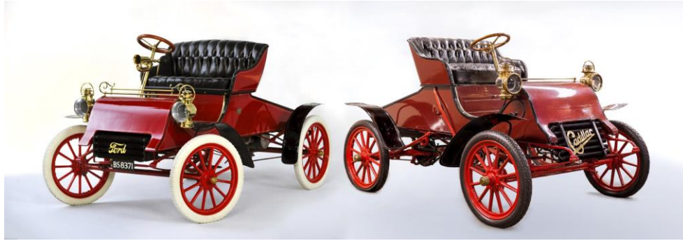
1903 Ford Model-A and 1903 Cadillac Model-A runabouts, exactly the same bodies, different engines.
